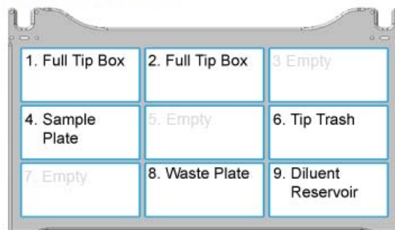
Figure Bravo deck layout for BenchCel 4R and 6R protocols (top view)
