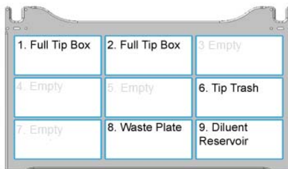
Figure Bravo deck layout for BenchCel 4R and 6R protocols (top view)
